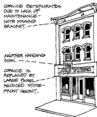
3. More Minor Facade Change
