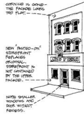
4. Storefront Remodeling - Facade Looks Cut in Half.
