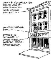
3. More Minor Facade Change
