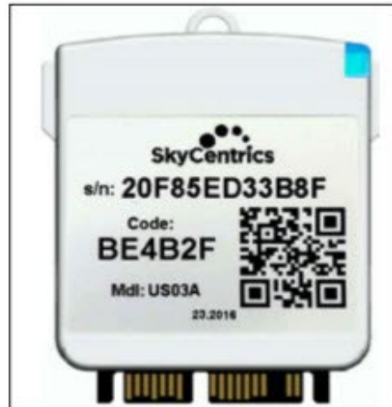
Figure 3: DC Form Factor Communications Module. Photo courtesy of SkyCentrics
