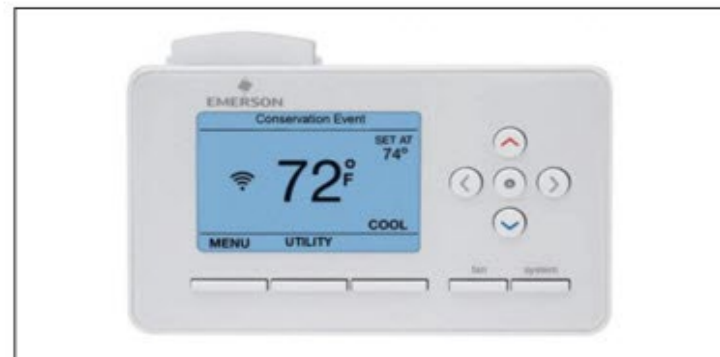
Figure 4: DC Communications Module Plugged into the Upper Left Corner of an Emerson Smart Thermostat. Photo courtesy of EPRI
