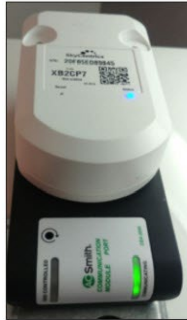
Figure 2: Photo of SkyCentrics AC Communications Module Connected to an A.O. Smith Water Heater. Photo courtesy of SkyCentrics
